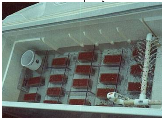
3 - Streamside incubator with Whitlock-Vibert boxes holding incubating eggs in an old freezer.
