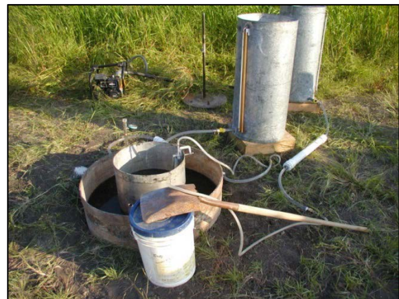
Track-mounted drill rig creating a bore hole for soil sampling and hydraulic conductivity testing (left), and ring permeameter test (right).
