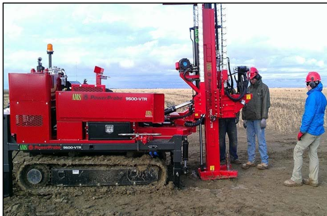
Track-mounted drill rig creating a bore hole for soil sampling and hydraulic conductivity testing (left), and ring permeameter test (right).
