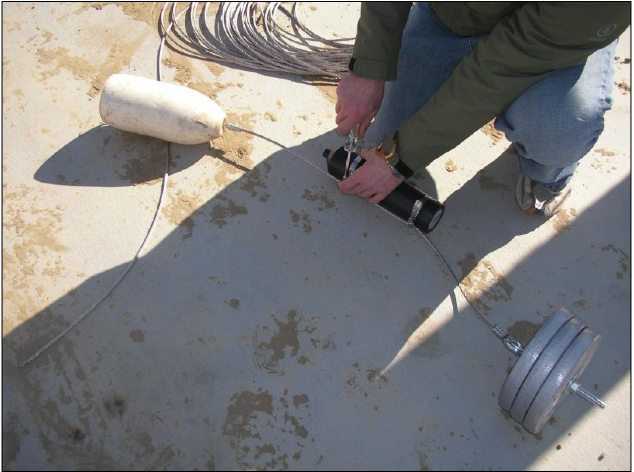
Figure 6: Vemco receiver with flat weights and buoy
