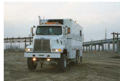
Typical CPT Rig
