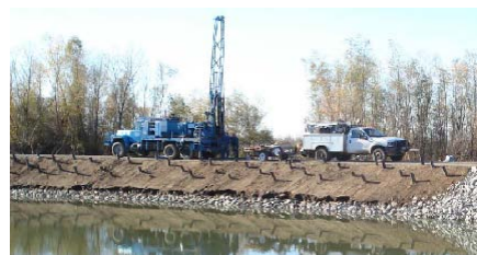
Drill Rig and support vehicle for HSA/SPT Borings
