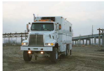
Typical CPT Rig
