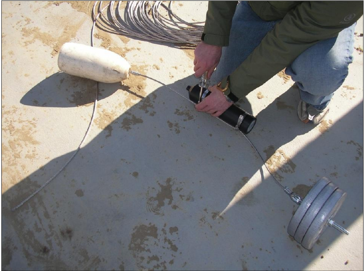
Figure 8: Vemco receiver with flat weights and buoy
