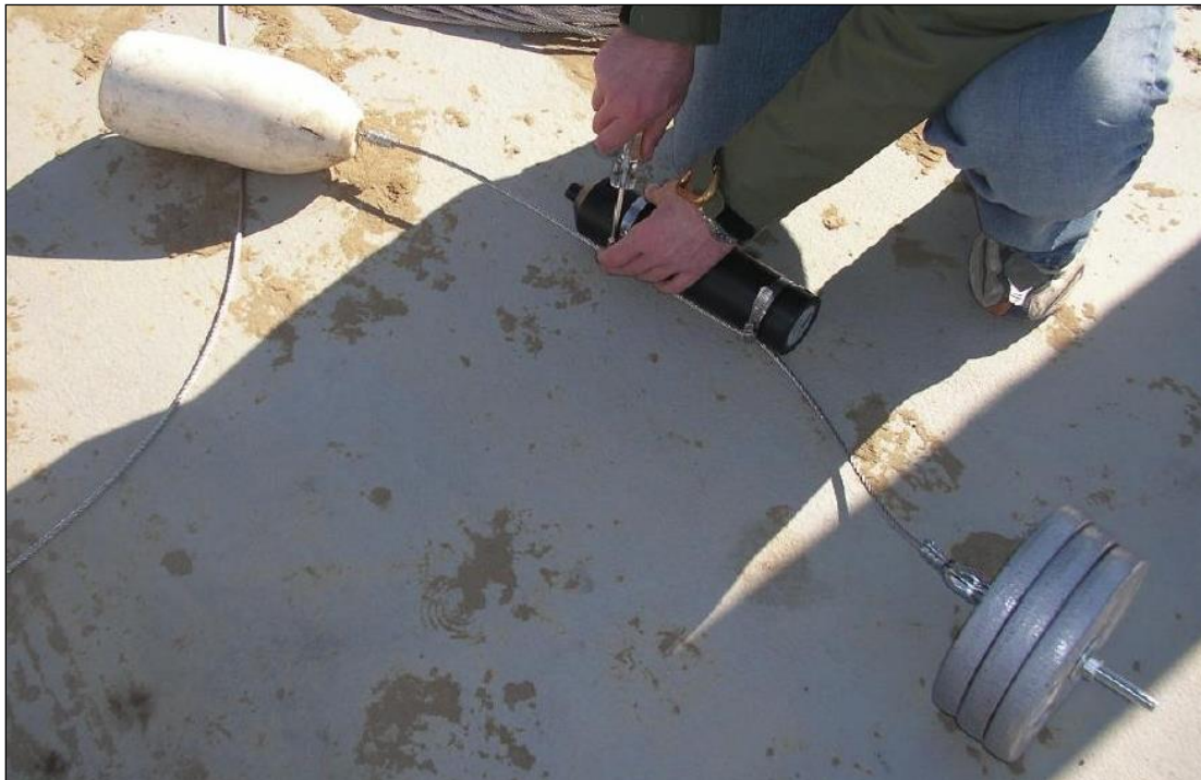
Figure 8. A single Channel Acoustic Monitoring Receiver (Vemco) Being Attached to a Stainless Steel Cable with Weights and Bouy. Stationary Receivers will be used to Track Movements of Adult fall-run Chinook Salmon in Reach 1 of the San Joaquin River
