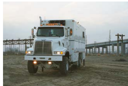
Typical CPT Rig
