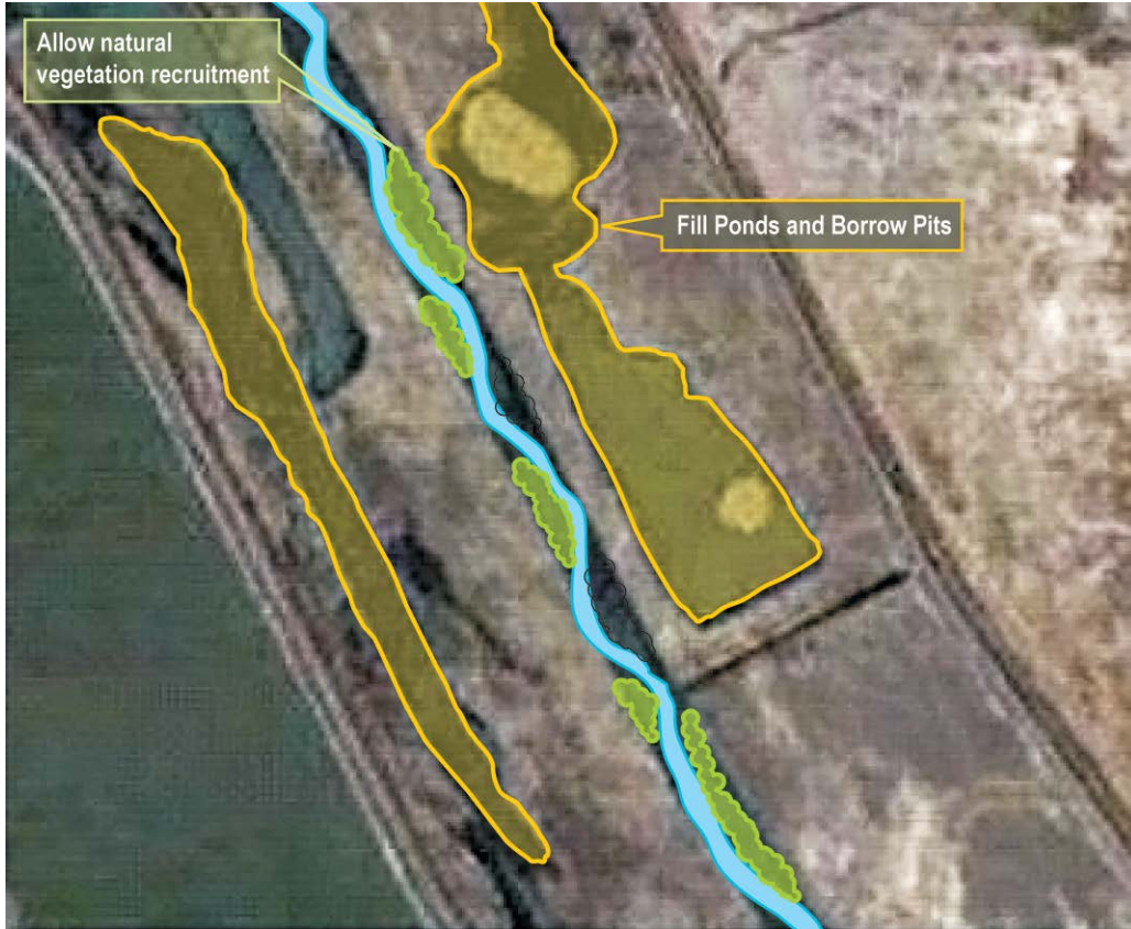
Figure 3-15. Alternative 3 – Example of Channel Excavation in the Eastside Bypass
