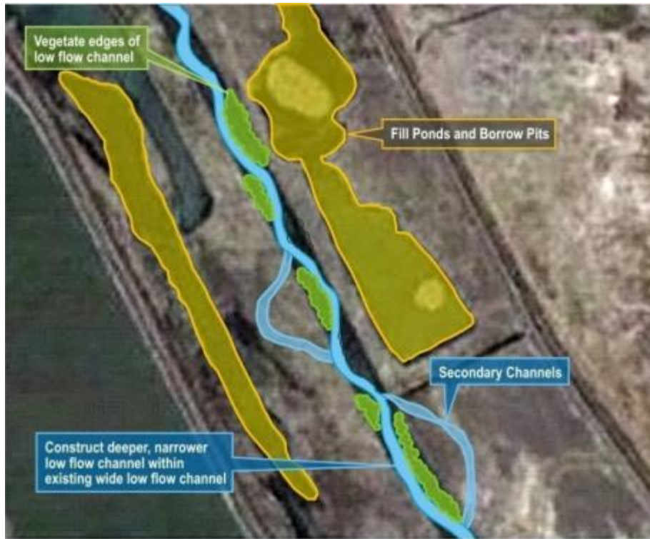
Figure 3-11. Alternative 2 – Example of Channel Excavation in the Eastside Bypass
