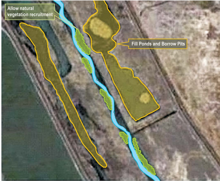
Figure 3-22. Alternative 4 – Example of Channel Excavation in the Eastside Bypass
