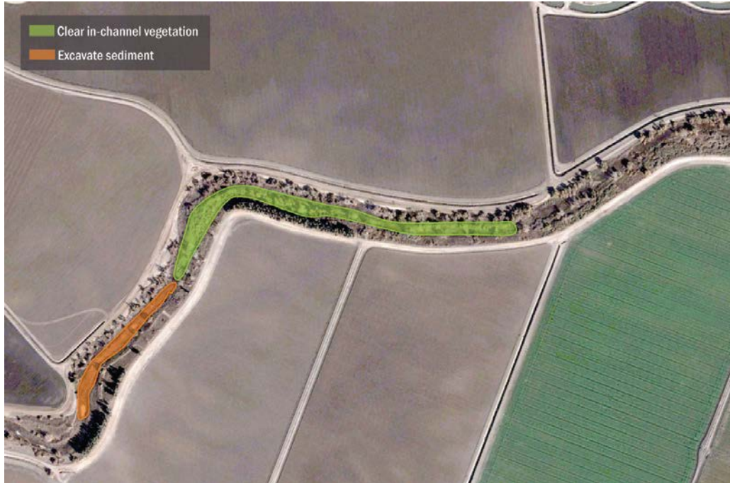
Figure 3-10. Alternative 2 – Example of Channel Excavation and Vegetation Clearing in the San Joaquin River
