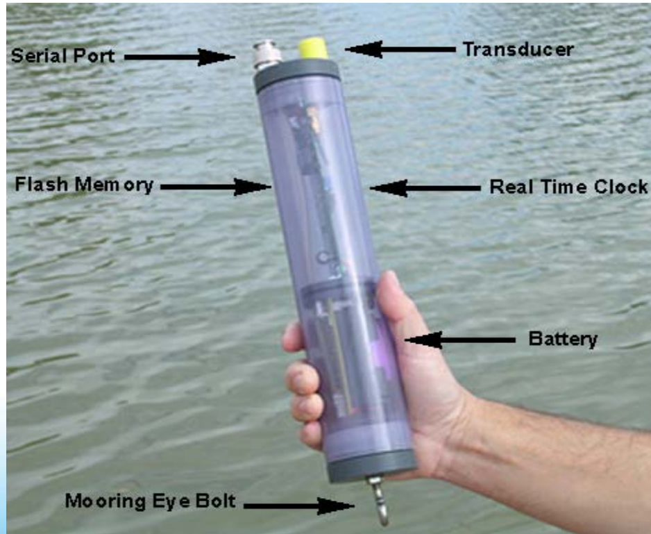
Stand-alone submersible ultrasonic receiver (Photo courtesy of Sonotronics Inc.)
