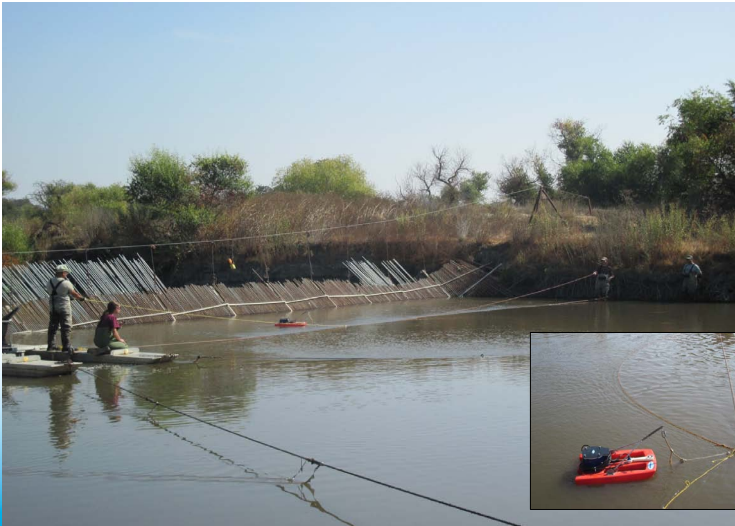
Measuring river velocity and bathymetry transects using an Acoustic Doppler Current Profiler
