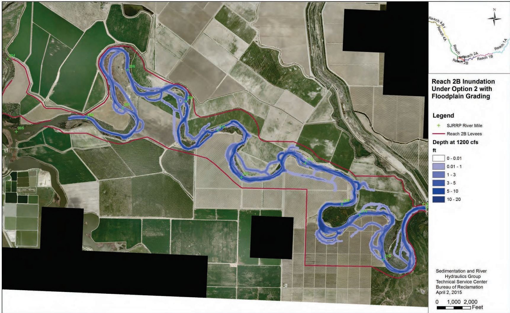
Figure C-42.—Depth of inundation for a flow of 1,200 cfs in Reach 2B under Option 2.
