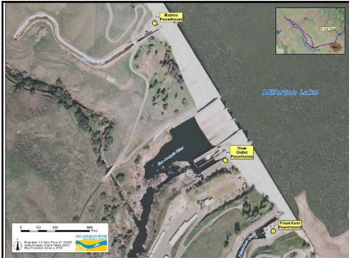
Figure 9. Hydropower Generation Facilities at Friant Dam
