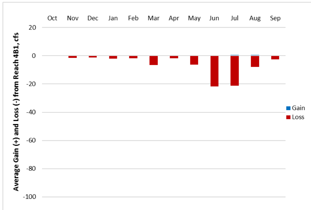
10 11 Figure F-44. 12 Simulated Average Monthly Gains/Losses from Reach 4B1 and the Middle 13 Eastside Bypass, based on May 1983 (Wet Year Type) Hydrologic Conditions 14 under Alternative 2
