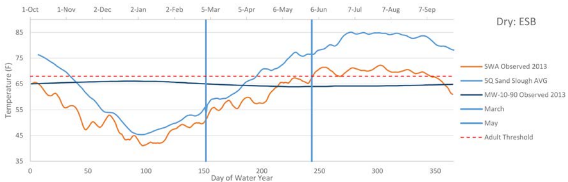
Figure 7-5. Surface Water and Groundwater Temperatures in the Eastside Bypass in a Dry Year
