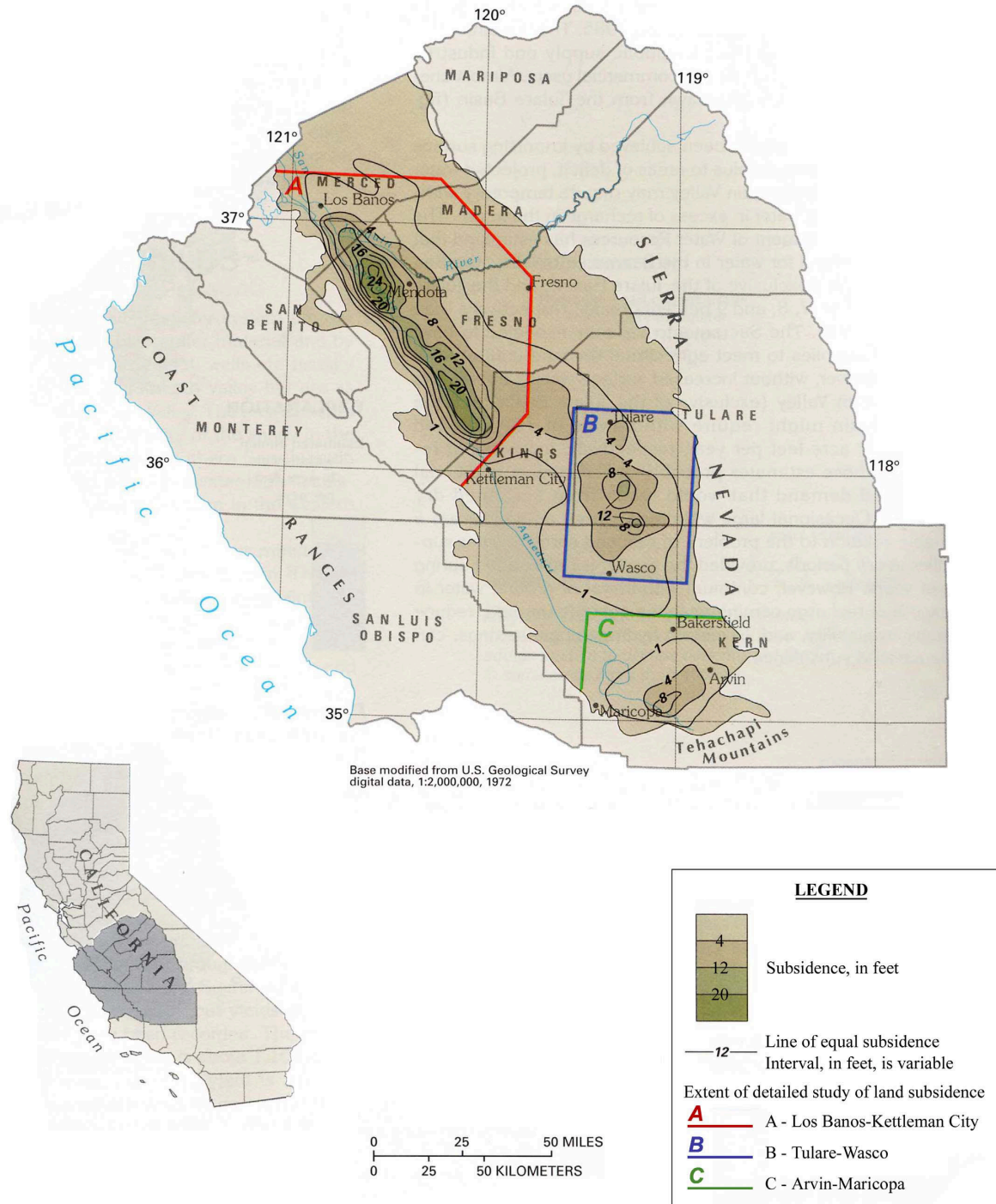
Figure 4-16. Zones of land subsidence in the San Joaquin Valley due to groundwater pumping. Land subsidence is most severe in the southern portion of the San Joaquin River corridor and Tulare Lake basin between Los Banos and Kettleman City. Modified from Ireland (1986).
