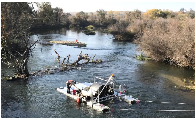
Figure 2. Rotary screw trap used to capture juvenile Chinook Salmon in the San Joaquin River, CA.
