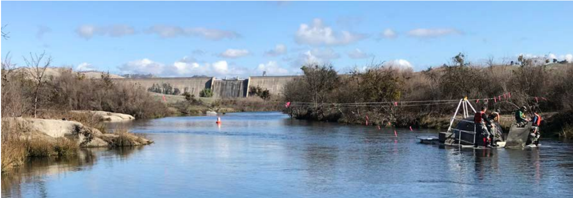
Figure 2. —Friant rotary screw trap attached to high line wire rope via snatch block and smaller diameter wire ropes (made apparent to recreationalists using pink flagging).
