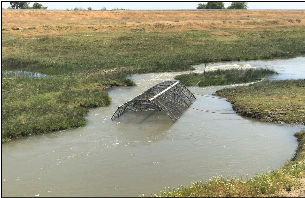
Figure 2. — Steel fyke trap used to monitor for adult spring-run Chinook Salmon ( Oncorhynchus tshawytscha ) in the San Joaquin River Restoration Program Restoration Area (Eastside Bypass trap location).
