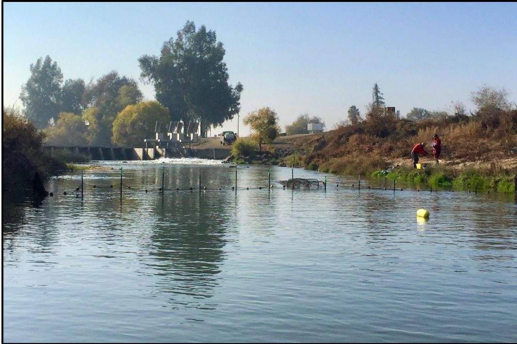
Figure 3. — Mesh fyke net erected downstream of the Sack Dam in the San Joaquin River Restoration Program Restoration Area to monitor for adult spring-run Chinook Salmon ( Oncorhynchus tshawytscha ).
