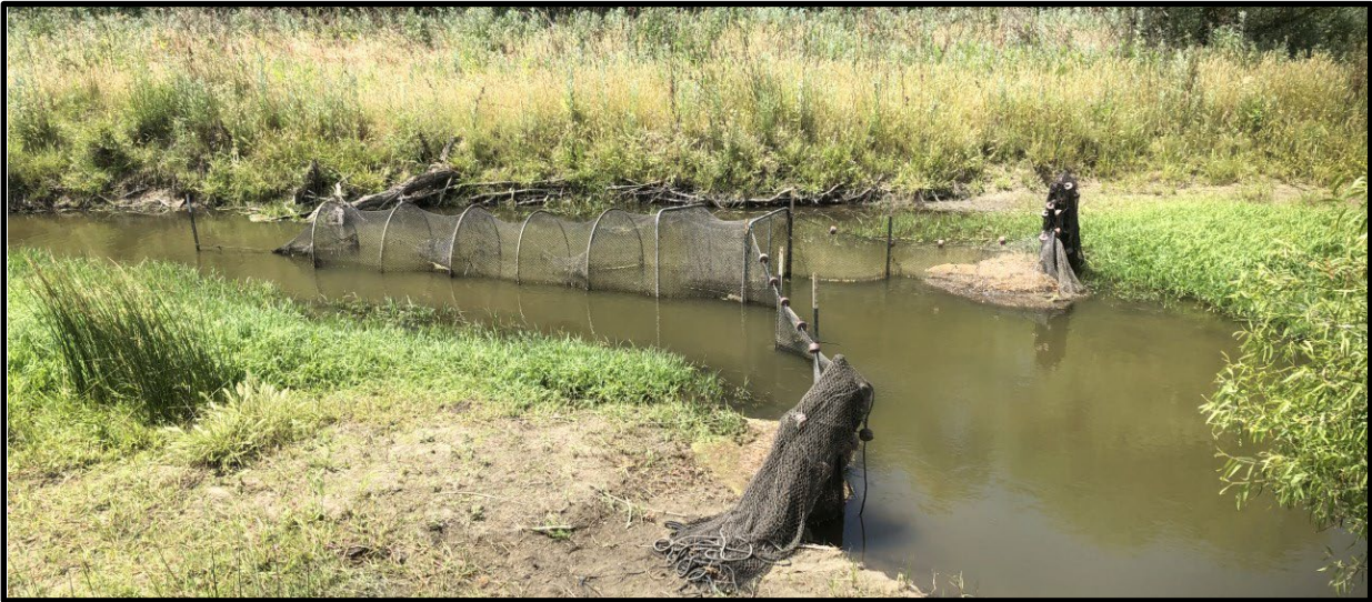
Figure 3. — Mesh fyke net used to monitor for adult spring-run Chinook Salmon ( Oncorhynchus tshawytscha ) at the Van Clief location in the San Joaquin River Restoration Program Restoration Area.
