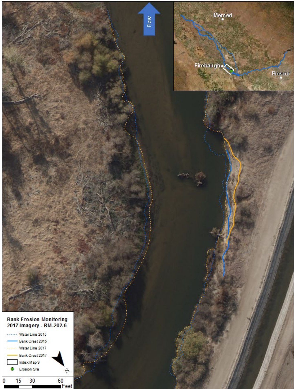
Figure 10 San Joaquin River Reach 3, RM 202.6; Threat Ratio 1.6, Threat Level: High; Index Map 9
