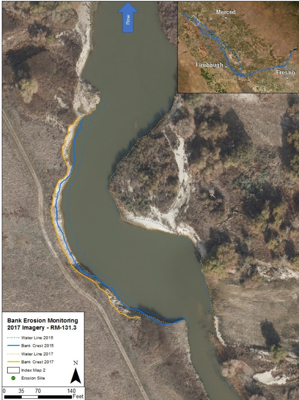
Figure 3-2. Example of a high threat erosion site in Reach 5
