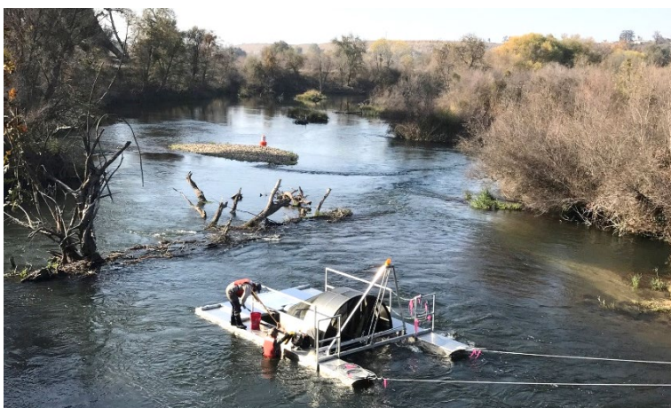
Figure 2. Rotary screw trap used to capture juvenile Chinook Salmon in the San Joaquin River, Calif.
