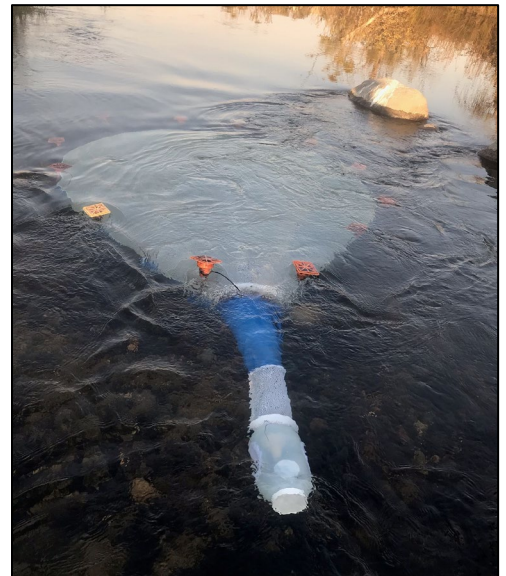
An emergence trap is used to assess egg survival and emergence rates from salmonid redds, or nests.
