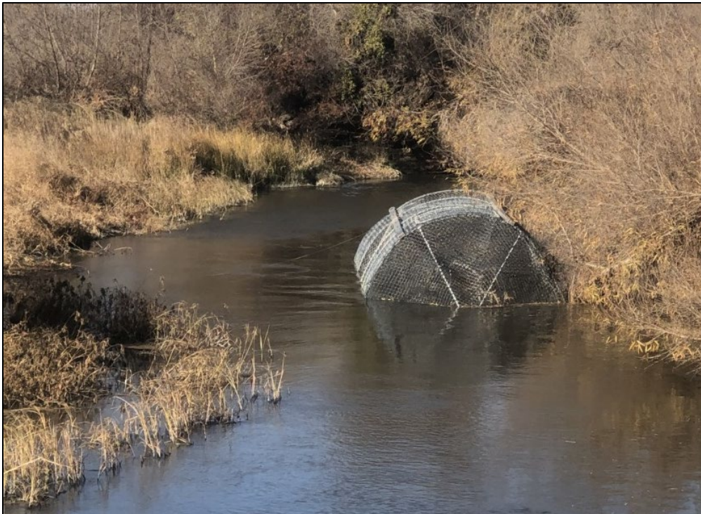
Figure A-2. Fyke trap monitoring, 2020-21 Steelhead Monitoring Plan, Mud Slough, Reach 5, San Joaquin River, CA.
