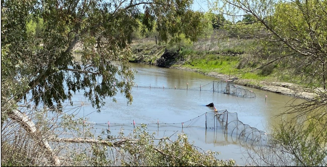
Figure 2. Deployed overlapping fykes net at Hills Ferry Barrier location, Reach 5 of the San Joaquin River Restoration Area. Note opening and v-shape of wing walls facing downstream.
