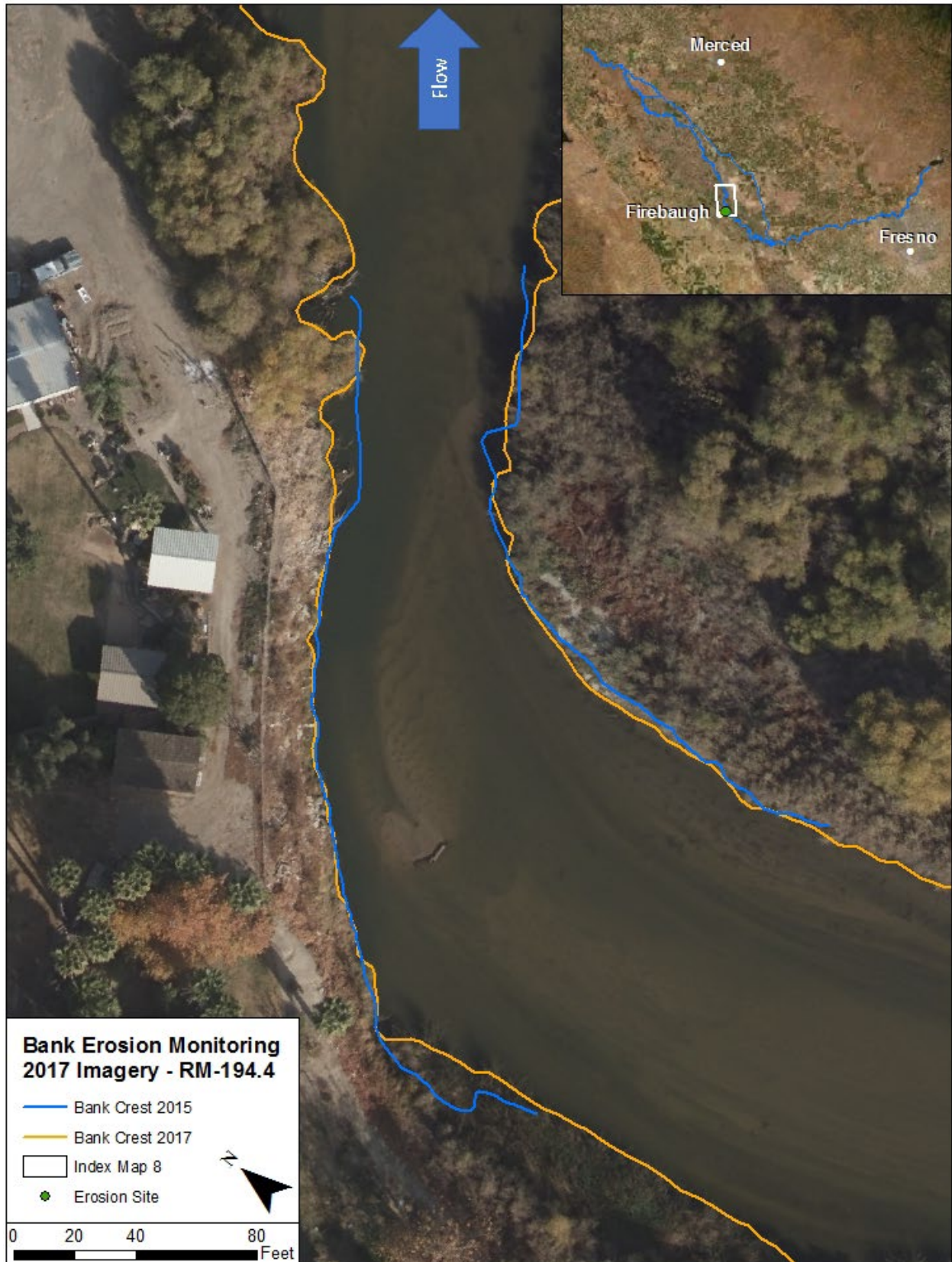
Figure 11 San Joaquin River Reach 3, RM 194.4, Threat Ratio 2.0, Threat Level: High, Index Map 8
