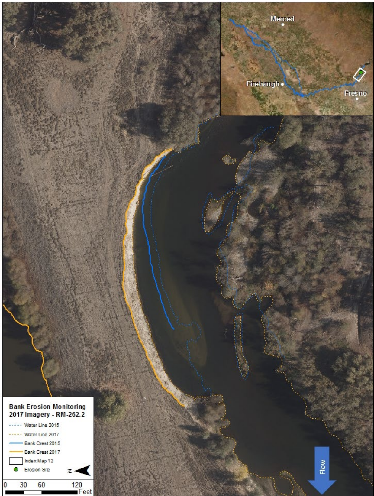
Figure 9 San Joaquin River Reach 1, RM 262.2; Threat Ratio 1.5, Threat Level: High; Index Map 12
