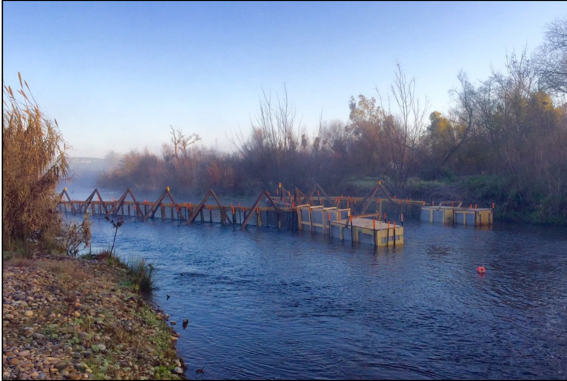
Figure 3.— Upstream looking image of weirs, diffuser box and capture boxes used to capture emigrating juvenile Chinook Salmon during the San Joaquin River Restoration Program's Juvenile Trap and Haul Program (San Joaquin River, CA).
