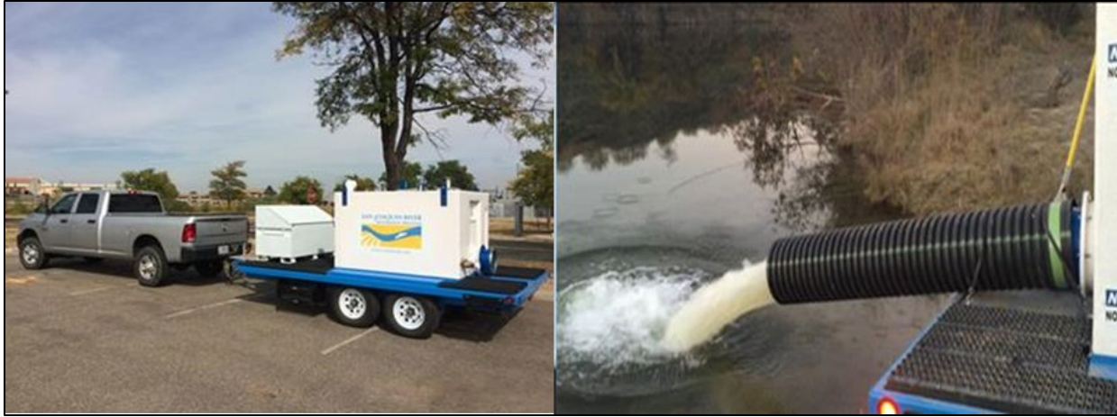
Figure 8.—Trailer-mounted haul tank (2,574-L; at left) and release method (at right) used by Bureau of Reclamation during the 2015 and 2016 Fall-Run Chinook Salmon Adult Trap and Haul Program.
