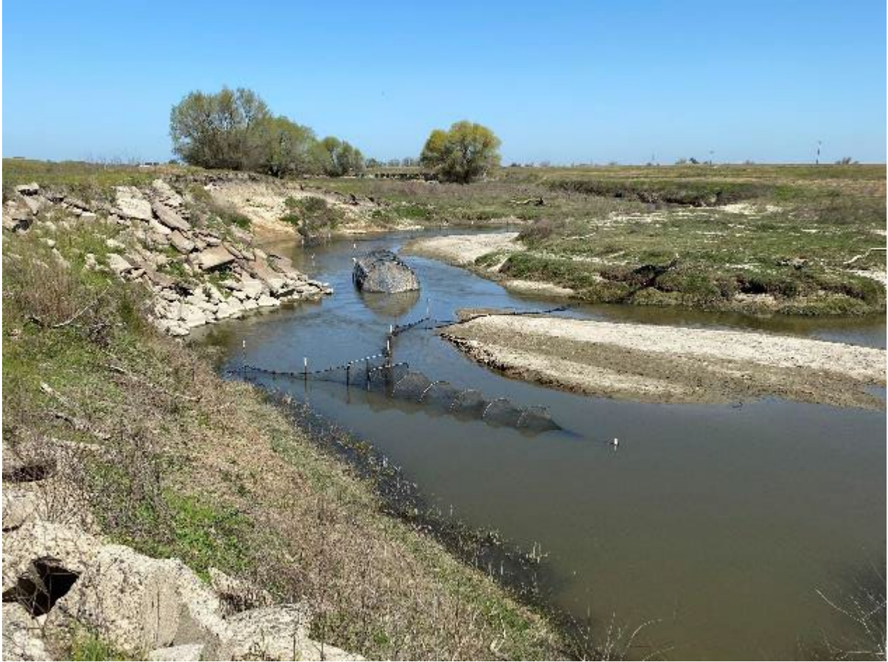
Figure A-2. — Sampling equipment (two fyke nets and one fyke trap pictured) immediately downstream of the Eastside Bypass Rock Weir at the Van Clief location (see Figure 1 for map) during 2021 San Joaquin River Restoration Program adult spring-run Chinook Salmon ( Oncorhynchus tshawytscha ) monitoring and trap and haul.
