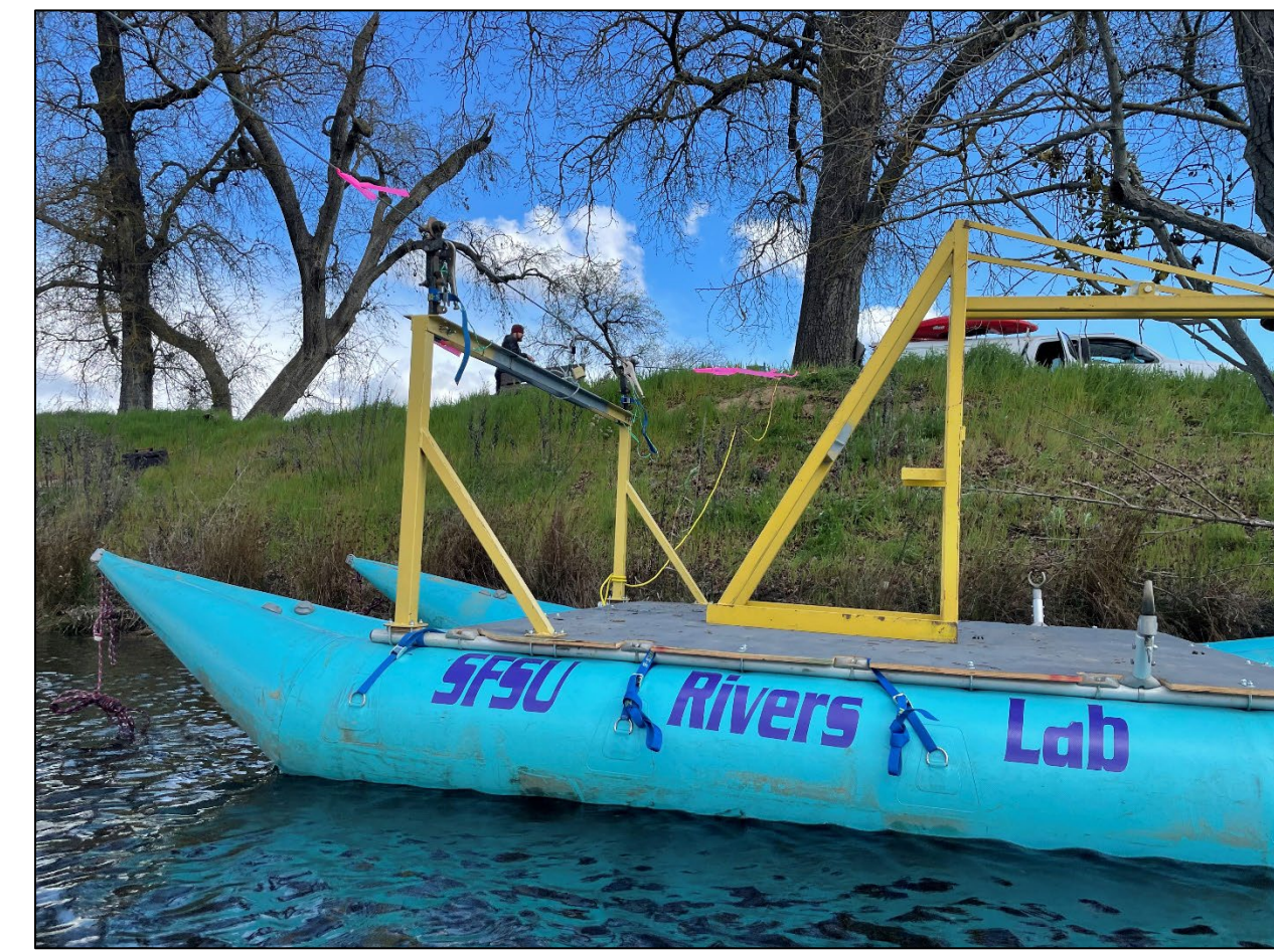
Figure 1. San Francisco State University (SFSU) Bray Rivers Lab cataraft. Cableway and towers allow lateral traversing across the channel and the crane boom lowers a bedload sampler into the channel.
