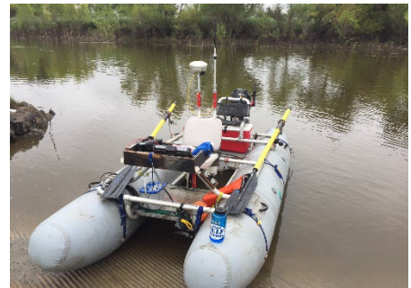
Shallow water boat for vessel-based bathymetry data collection.
