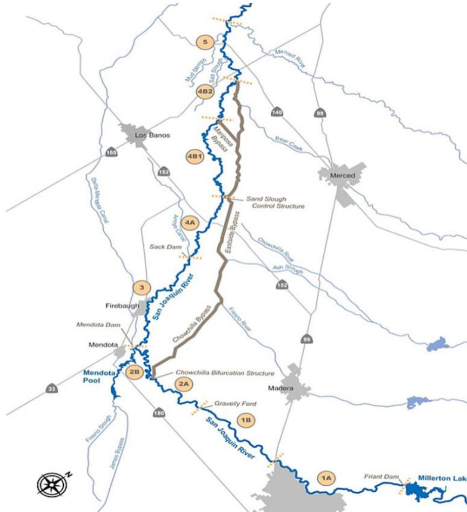
Figure 1.—Map of the San Joaquin River Restoration Area and associated Reaches. The area encompasses the San Joaquin River below Friant Dam to the confluence of the Merced River. The yellow circles identify the associated Restoration Reach, and the dashed lines identify the boundary between reaches.
