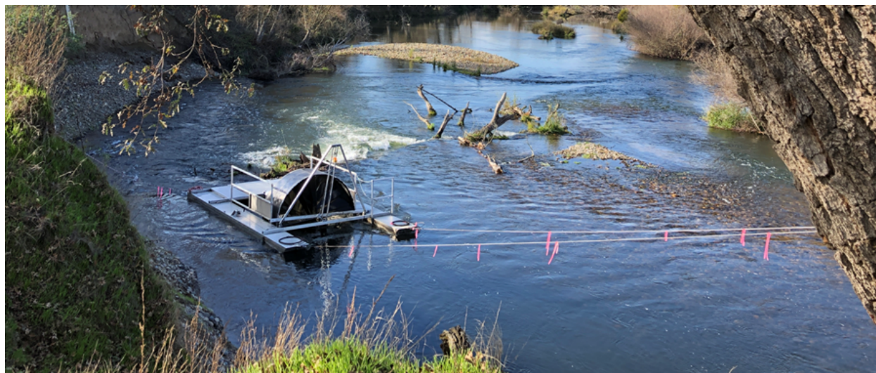
Figure 2.— Owl Hollow rotary screw trap attached to high line wire rope via snatch block (not visible) and smaller diameter wire ropes (made apparent to recreationalists using pink flagging). Lateral rope, connected to shoreline, on downstream side of trap prevents excessive swaying.
