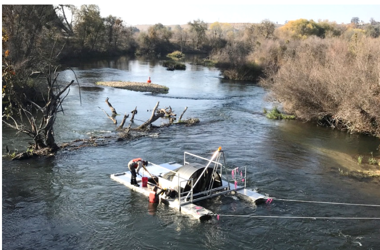
Figure 2. Rotary screw trap used to capture juvenile Chinook salmon in the San Joaquin River, California.
