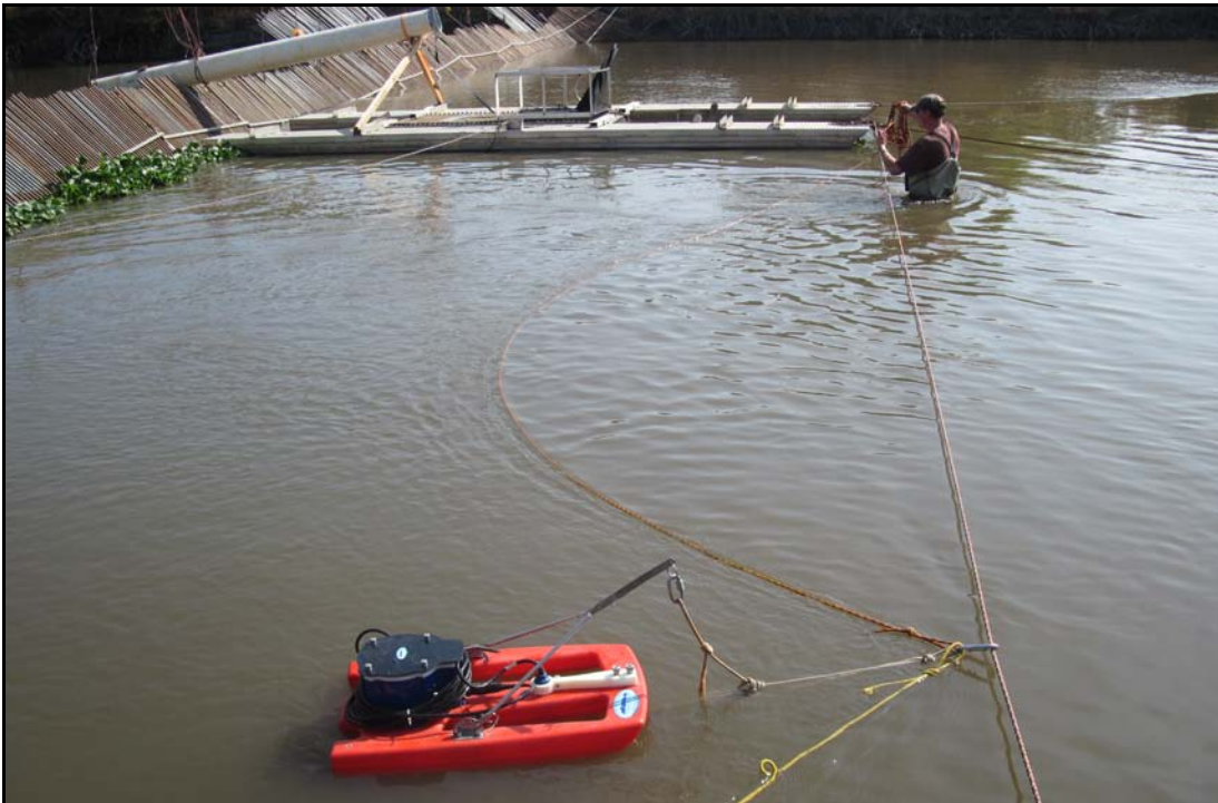
Figure 6.—Measuring river velocity and bathymetric transects utilizing the Acoustic Doppler Current Profiler.
