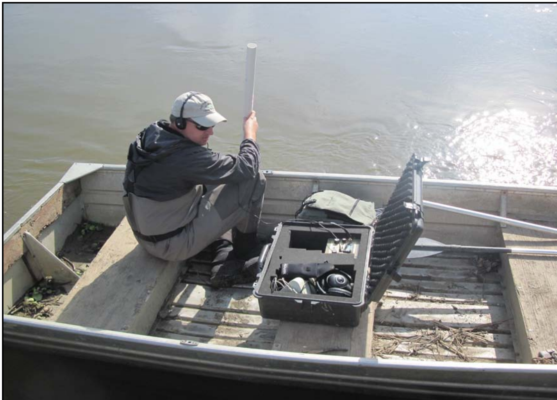
Figure 9.—Manual tracking of an acoustically-tagged Chinook salmon using a Sonotronics USR-5W wide band receiver with DH-4 directional hydrophone.
