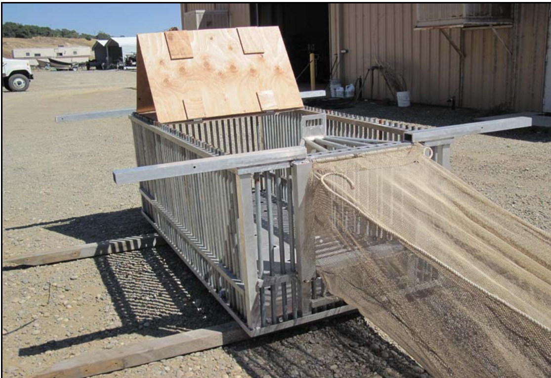
Figure 4.—Fish trap retrofitted to the Hills Ferry Barrier sliding pipe weir design that consisted of a 1-m-wide x 2-m-long x 1-m-high (3.28-ft-wide x 6.56-ft-long x 3.28-ft-high) box frame with 2.5-cm (1-in) bars spaced at 2.5 cm (1 in) and a funnel opening to deter escapement. The net entrance led from the weir to the trap.
