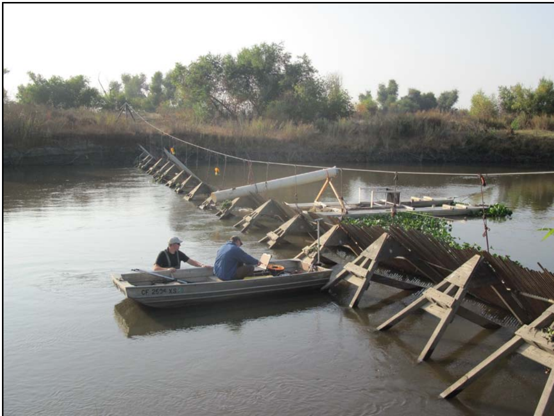
Figure 5.—River-wide transects were recorded along the barrier to monitor scouring and passage issues along with fish behaviors using a DIDSON camera affixed to a transom mount of a jon boat and manually maneuvered across the channel directly adjacent the barrier.
