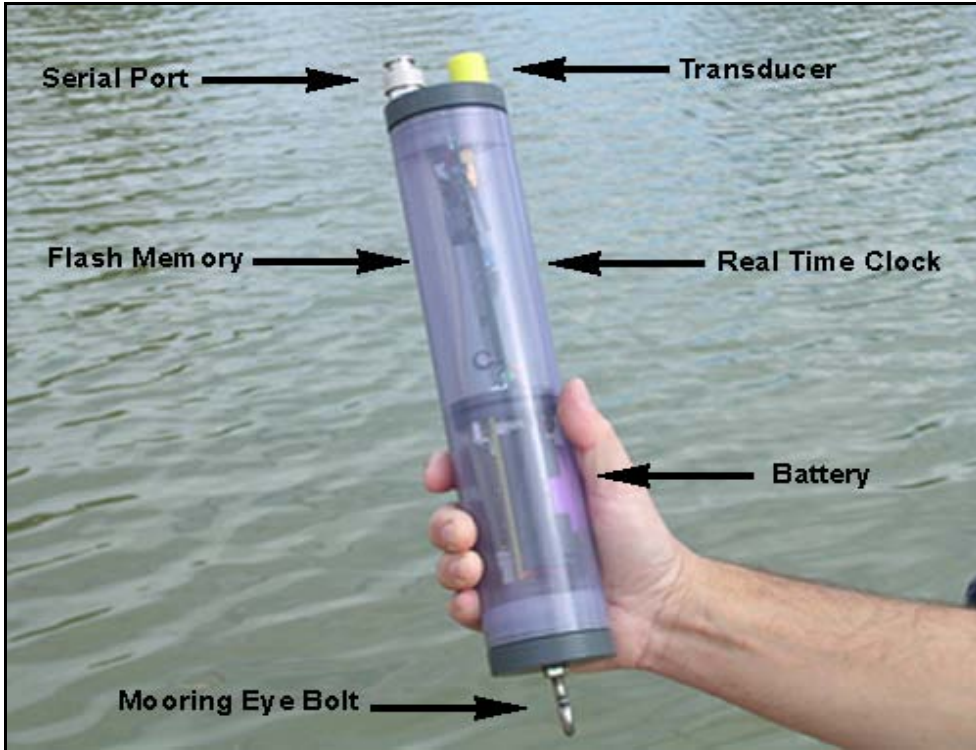
Figure 10.—Stand-alone submersible ultrasonic receiver (Photo courtesy of Sonotronics Inc.).
