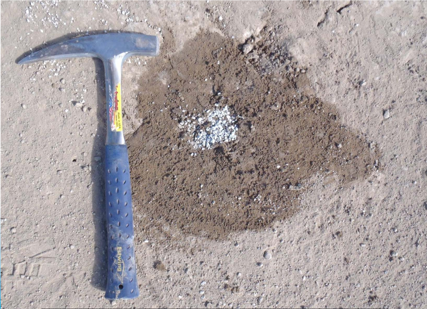
Completed CPT hole backfilled with granular bentonite
