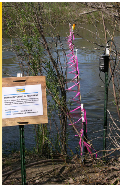
A PIT tag array in the San Joaquin River for fish monitoring
