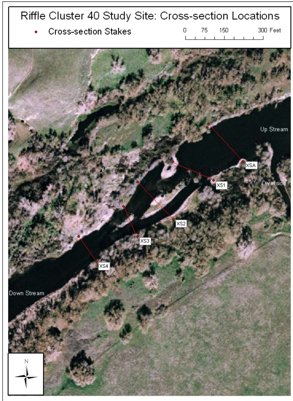
1 2 Figure 5-3: Riffle Cluster 40 study site's staked cross-sections XSA, XS1, XS2, XS3, 3 and XS4. 4
