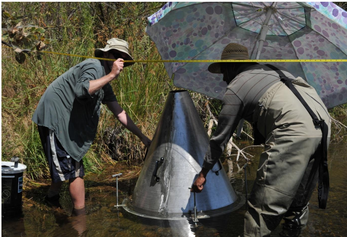
Figure B-30: Bed photography surveying using the photocone device. The yellow stretched tape is used to note each photograph's position along the cross-section. The umbrella is used to block light from entering both around the edges of the cone as well as into the hole behind the camera. Two people are needed to carry and hold the photocone in position while the third person takes photographs and records notes. Note the size of the photocone relative to the viewing bucket shown in the lower left corner of this figure.
