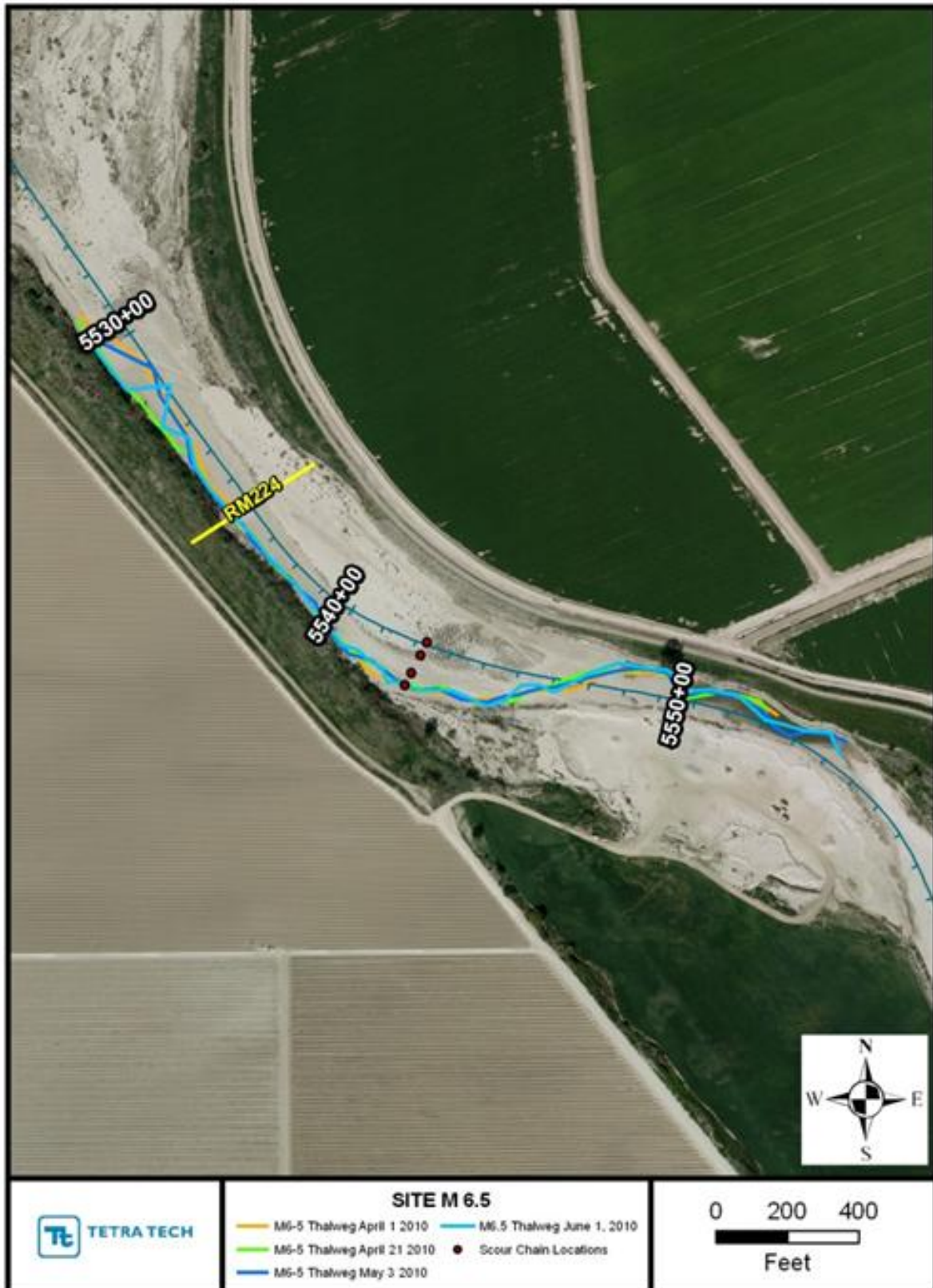
Figure B-19. Plan view showing the location of the thalweg during the spring 2010 bathymetric surveys at M6.5
