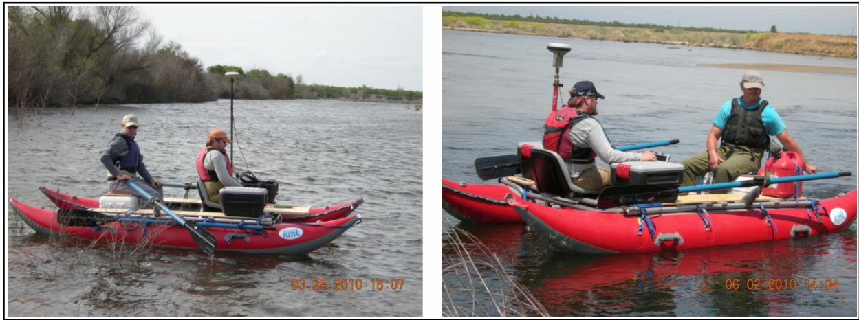
Figure B-17. Cataraft equipped with echo-sounder and survey-grade GPS rover
