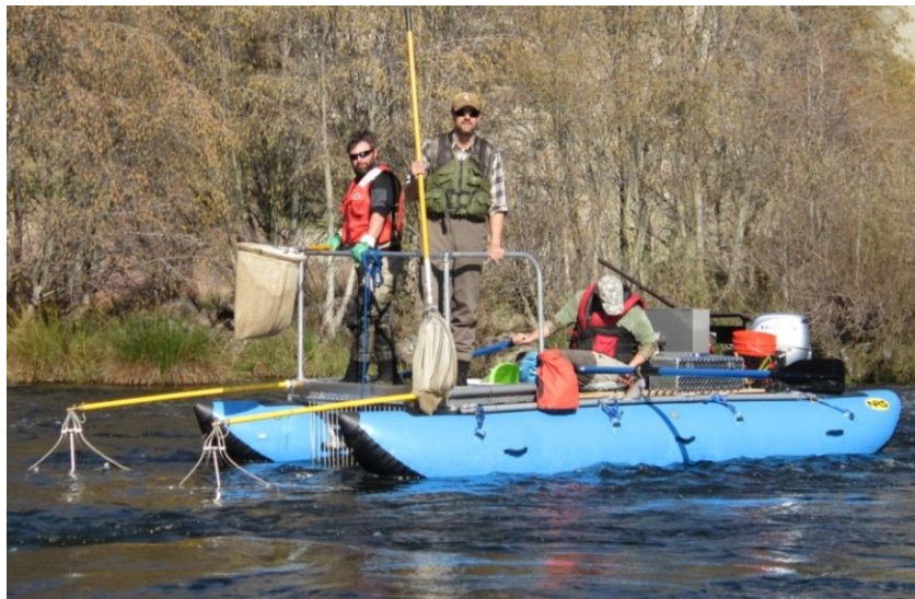
Figure 4. —Electrofishing raft and crew. Note extended boom array (ring anodes with vertically hanging cables not visible) and vertical cathode array (attached to the crew deck on the bow).
