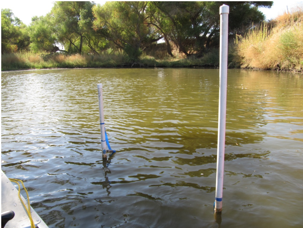
Figure A-21: SJR 199 downstream pool sensor arrays looking upstream.
