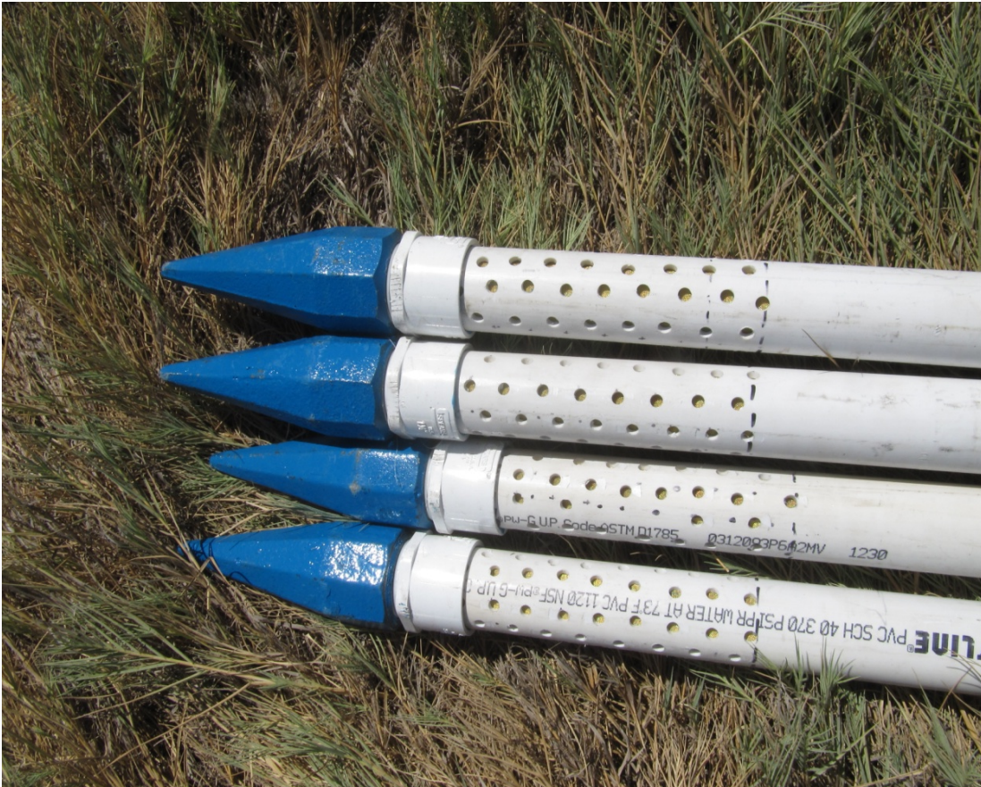
Figure 4: Screened bottom sections of sensor array piezometers
