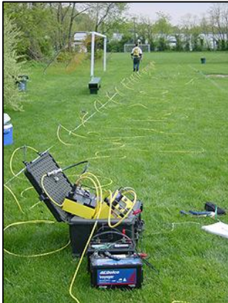
Figure: A typical arrangement of resistivity equipment
