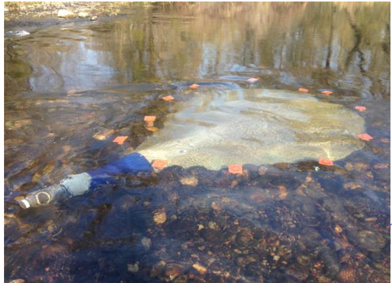
Figure 1: Emergence trap placed over redd in Reach 1 of the San Joaquin River during 2014.
