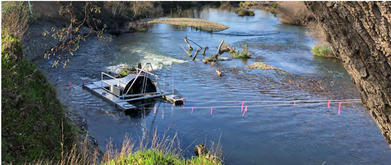
Figure 2. —Owl Hollow rotary screw trap attached to high line wire rope via snatch block (not visible) and 10 mm-diameter wire ropes (made apparent to recreationalists using pink flagging). Lateral rope, connected to shoreline, on downstream side of trap prevents excessive swaying. Photo credit: Bureau of Reclamation.
