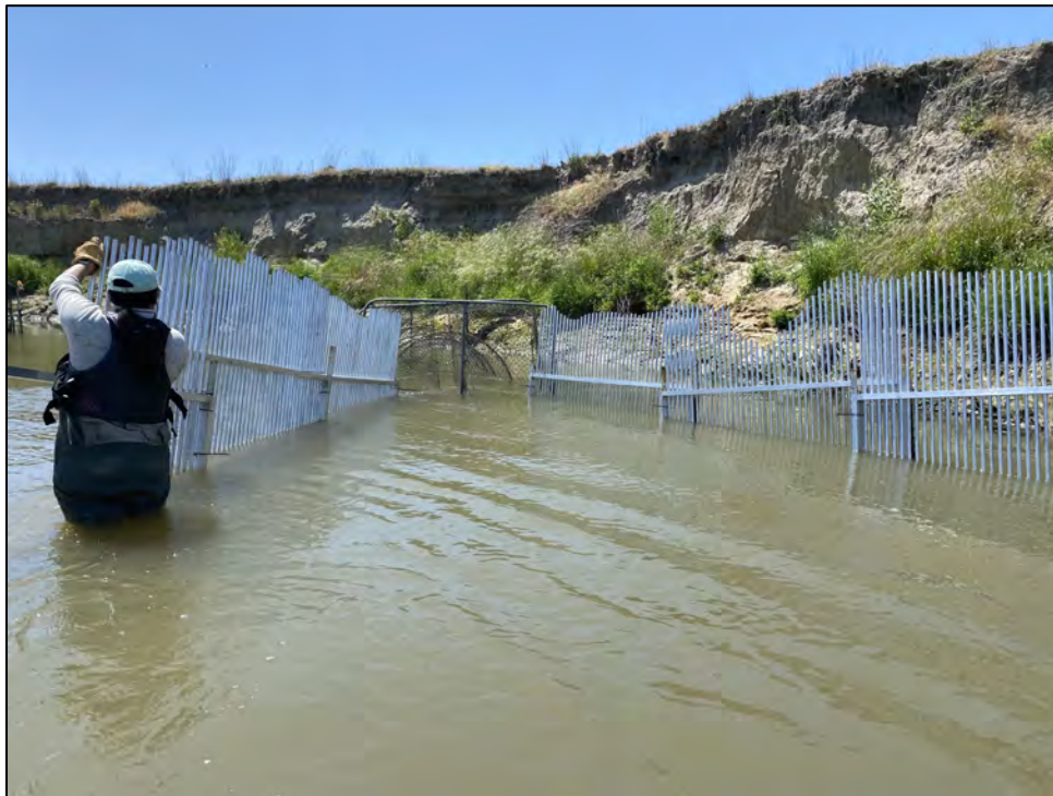
Figure 3. — Panel weir with fyke net used to monitor for adult spring-run Chinook Salmon ( Oncorhynchus tshawytscha ) at the San Joaquin River Van Clief location in the San Joaquin River Restoration Program Restoration Area.
