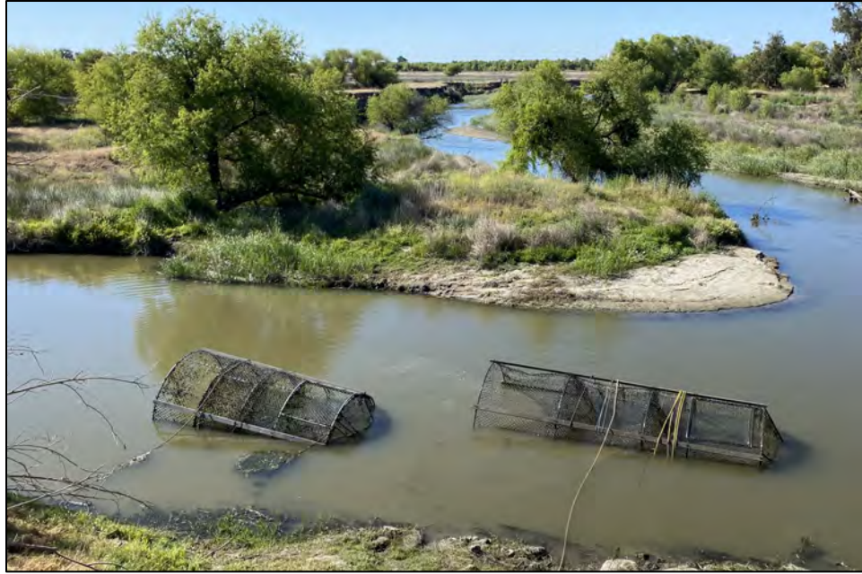
Figure 2. — Series of steel fyke traps used to monitor for adult spring-run Chinook Salmon ( Oncorhynchus tshawytscha ) in the San Joaquin River Restoration Program Restoration Area (Hills Ferry location).
