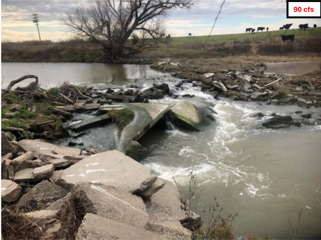
Figure 3. Photograph Date 3.10.2020 10:13. QA/QC data: EBM: 82 cfs daily avg, SJS: 122 cfs daily avg. C. Moore estimate approx. 90 cfs.
